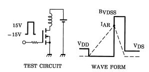
$$\begin{aligned} &R_G = 25~\Omega \\ &V_{DD} = 90~V,~L = 16.8~mH \end{aligned} \quad E_{AS} = \frac{1}{2} \cdot L \cdot I^2 \cdot \left( \frac{B_{VDSS}}{B_{VDSS} - V_{DD}} \right)$$
